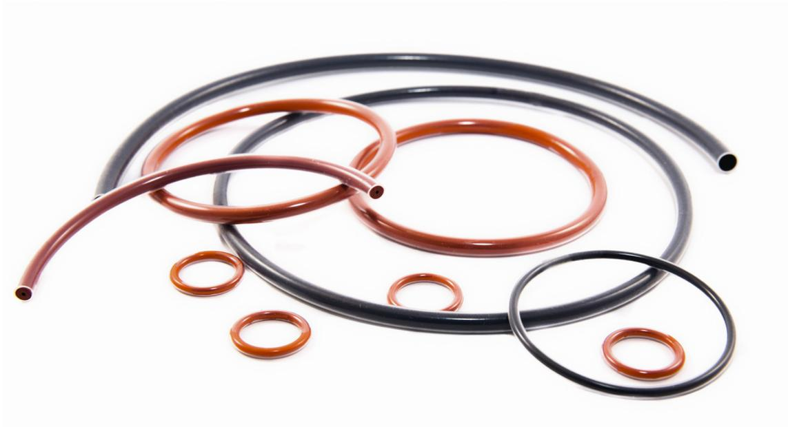
An encapsulated O-ring comprises of an elastomer core which has been seamlessly encapsulated in a jacket of Teflon® fluoropolymer. The core is either Viton® (FKM), Silicone (VMQ) or EPDM, and the jacket FEP or PFA.
