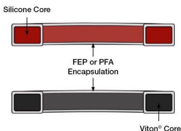
The chemical resistance of the jacket means that it can be used to seal a number of many different mediums eliminating the need for different compounds to be used.
