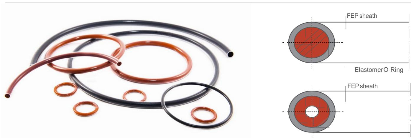
An encapsulated O-ring comprises of an elastomer core which has been seamlessly encapsulated in a jacket of Teflon<sup>®</sup> Fluoropolymer. The core is either Viton<sup>®</sup> (FKM), Silicone (VMQ) or EPDM, and the jacket FEP or PFA.
