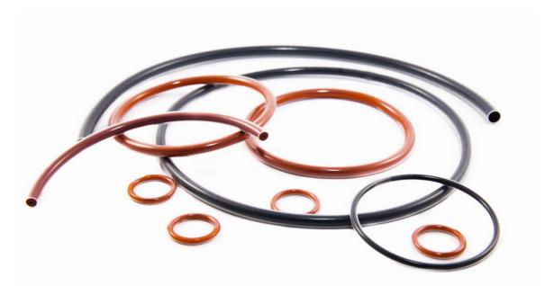
An encapsulated O-ring comprises of an elastomer core which has been seamlessly encapsulated in a jacket of Teflon® fluroropolymer. The core is either Viton® (FKM), Silicone (VMQ) or EPDM, and the jacket FEP or PFA.
